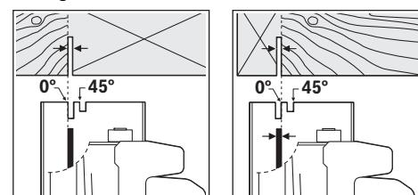
The 0° cutting mark **9** indicates the position of the saw blade for right-angled cuts. The 45° cutting mark **10** indicates the position of the saw blade for 45° cuts.
